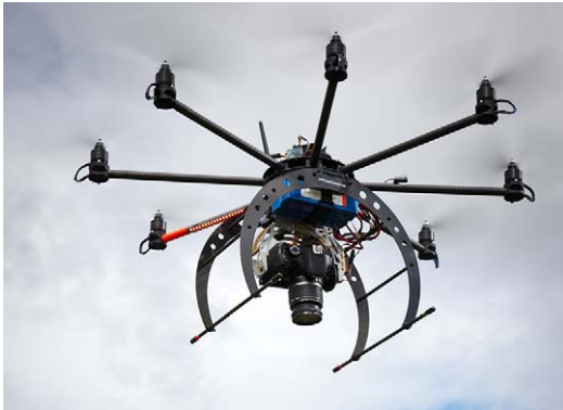
Figure 3. The remote controlled UAV OktoKopter equipped with digital camera and GPS.
