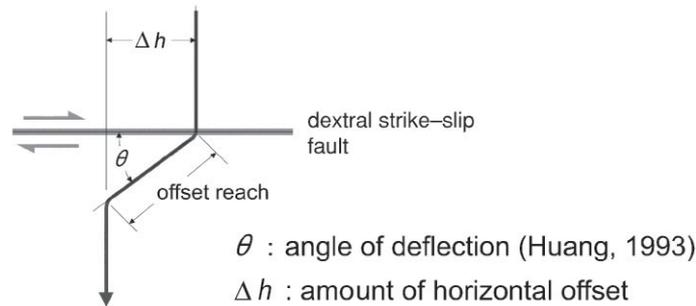
Figure 1. Terminology of an offset channel
