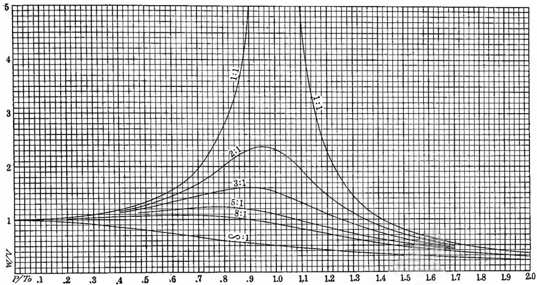
FIG. 47. — Magnifying power of linear displacements.
