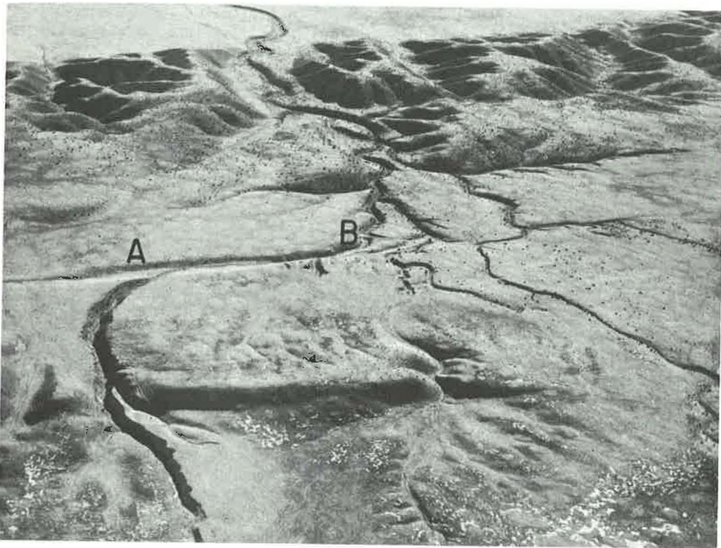
Figure 4.--Oblique view looking southwest across the San Andreas fault zone, Carrizo Plain area. Note multiple fault traces and deflection of streams at most active strand (second from bottom). The largest deflection, from A to B, is about 700 feet.
