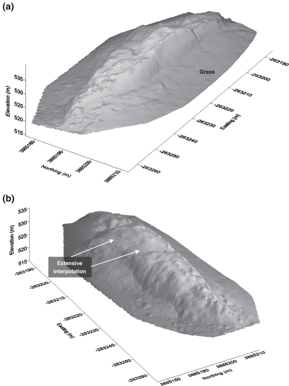
**Fig. 14.** Oblique, hill-shaded views of the final SfM DEM Cwm Cau bedrock ridge, showing the (a) south and (b) north faces. Areas of low point density resulted in extensive interpolation across elevated sections. Data transformed to the UK Ordnance Survey National Grid coordinate system (OSGB36 datum).
