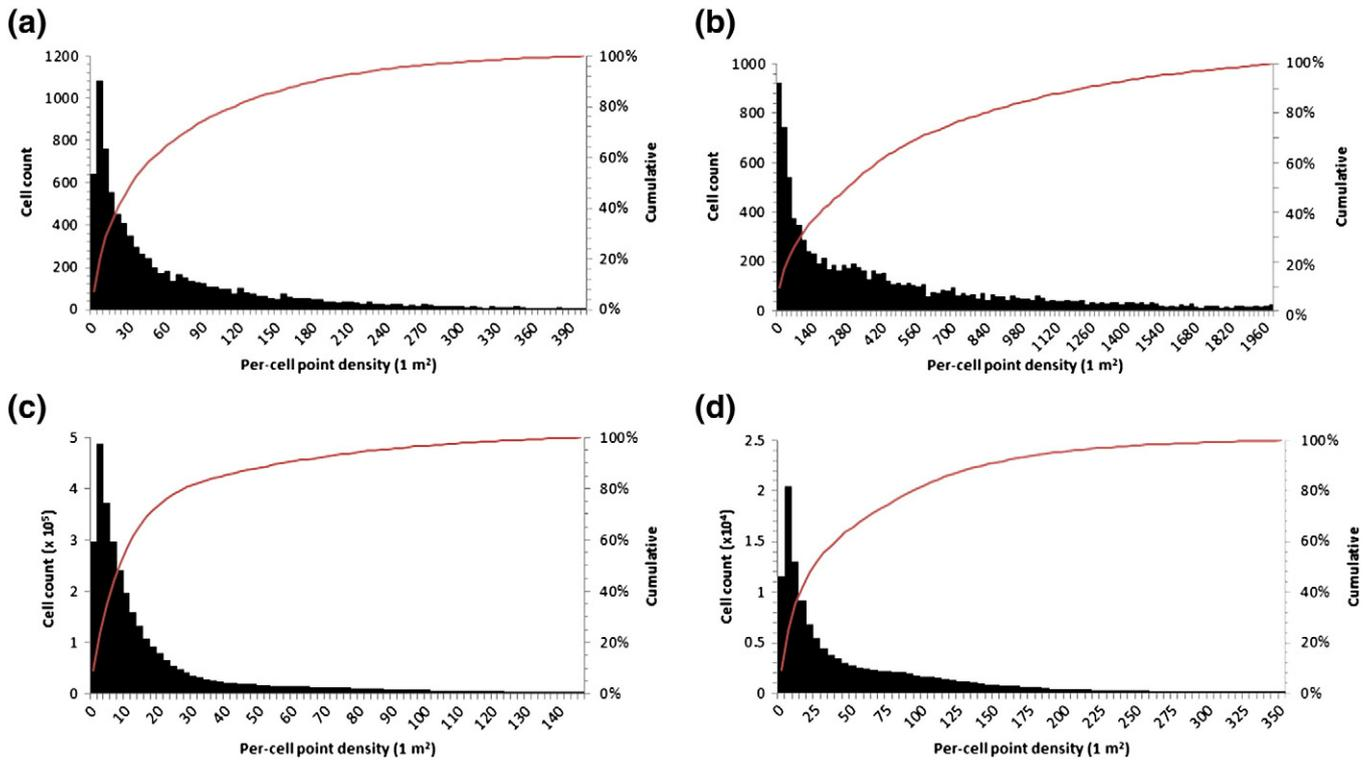
**Fig. 8.** Per-cell point density frequency distribution plots. (a) Constitution Hill SfM DEM. (b) Constitution Hill TLS DEM. (c) Dig Tsho SfM DEM (note: upper limit of x axis manually truncated at 150 points per m<sup>2</sup> to preserve histogram form; refer to Fig. 12b for complete range of density values). (d) Cwm Cau SfM DEM.
