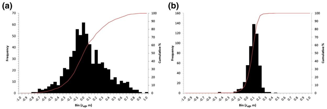
**Fig. 10.** Local scale (20 m<sup>2</sup>)  $z_{diff}$  frequency distribution data for an area with (a) dense vegetation cover (DV), and (b) vegetation-free (VF). As anticipated, elevation differences in the absence of vegetation are considerably lower. See Fig. 7 for locations of DV and VF.
