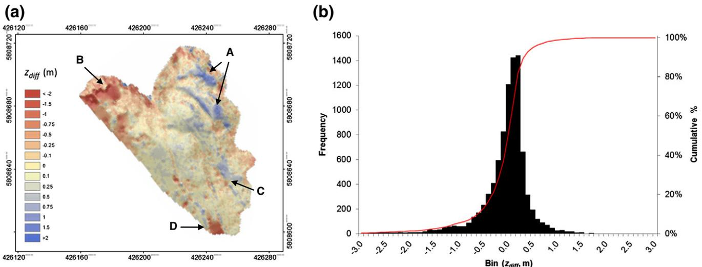
**Fig. 9.** DEM of difference results (TLS – SfM). (a) Spatial representation of the  $z_{diff}$  frequency distribution. Data georeferenced to UTM Zone 30N coordinate system. (b)  $z_{diff}$  frequency distribution. A: The headwall at the highest point of the surveyed area; B: near-vertical cliffs; C: dense vegetation cover; D: interpolation error.
