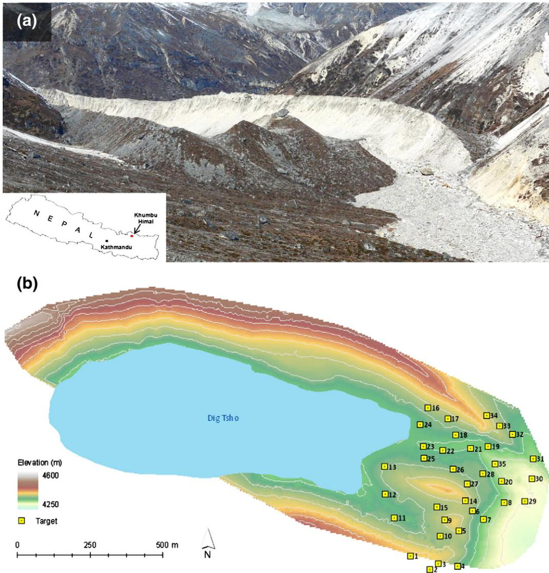
**Fig. 11.** Dig Tsho glacial lake. (a) View towards the terminal moraine complex at Dig Tsho, Khumbu Himal, Nepal. A large breach, produced by a glacial lake outburst flood is clearly identifiable to the right of the photograph. (b) Spatial extent of SfM reconstruction. GCP locations also shown. (Photo: M. Westoby).
