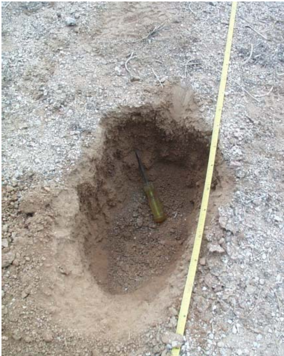
Figure 3: Regolith thickness measurements were made in pits like this. We used the shovel or screwdriver to determine the depth of the largest change in induration (screwdriver tip). Sometimes we would note a second level where the induration changed (at the base of the hole in this picture).
