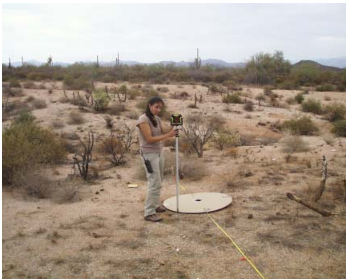
Figure 1: Surveying along the burnt transect. We used the 1 m template to better control the curvature point survey. We sampled at the central point for regolith and grain size.
