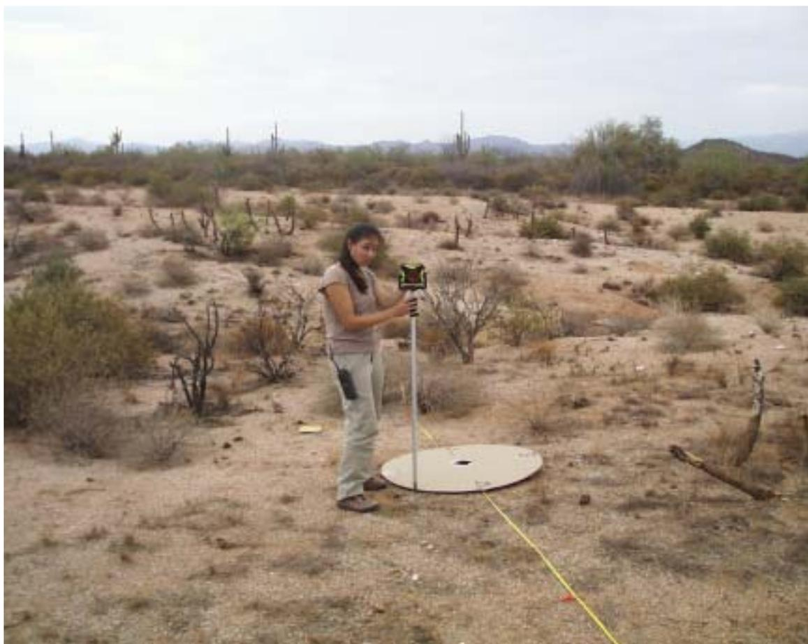
Figure 1: Surveying along the burnt transect. We used the 1 m template to better control the curvature point survey. We sampled at the central point for regolith and grain size.
