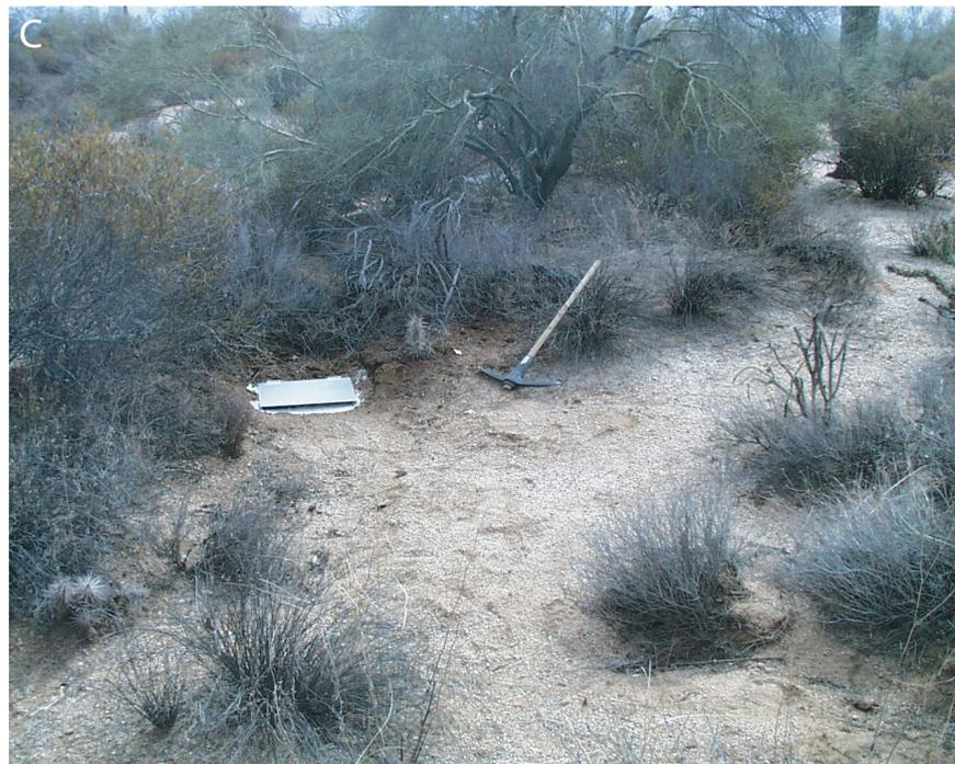
Figure 7. Sediment trap installation. A) Basic design and situation within drainage basin. B) view of open trap with cement lip. C) Closed trap at narrow portion of shallow channel.
