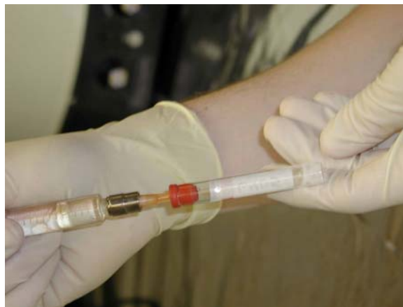
Fig. 11 Needle piercing through septum, then plunger pushed to expel acid
