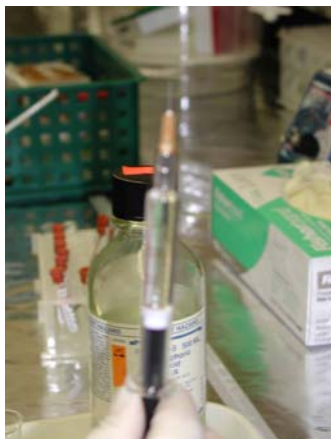
Fig. 10 Syringe turned upside-down and plunger pushed in to expel air bubble.
