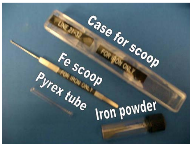
Fig. 2 Tools necessary to load Fe-catalyst into the graphitization line.
