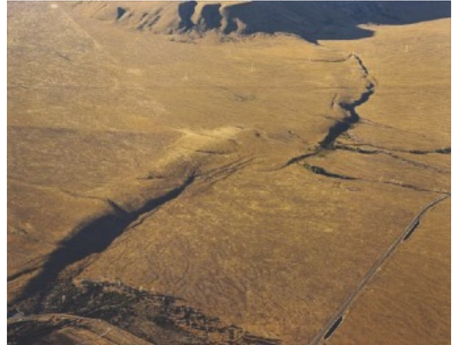
Ostler fault, New Zealand (NZ geological survey). Similarities include scarp morphology, hanging wall extension and folding, wrinkles in front of scarp, and occurrence of one late Holocene earthquake.
